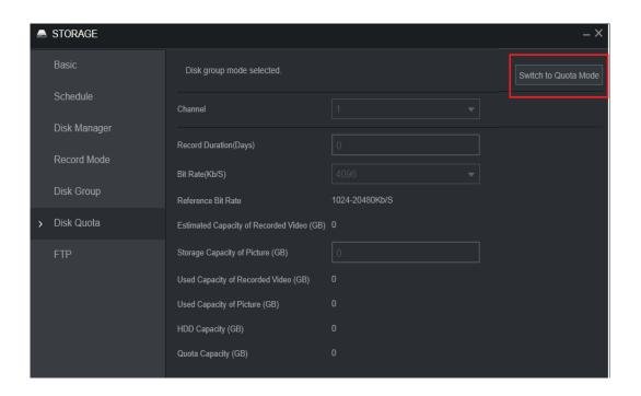
ii. Quota management allows storage capacity to be set by channel, and videos and images can be configured separately, and the remaining configurable space is automatically calculated.
