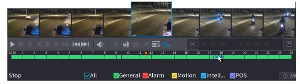
**iii.** Multi-channel dragging with picture browsing in iframe. This feature supports prompting a pop-up window for thermal event linkage. When playing back videos, you can drag the vertical orange line on the time bar to rapidly view the playback in iframe format.
