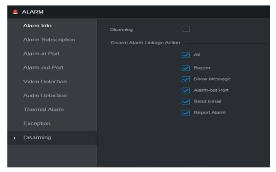
ii. The **Live** interface supports one-click disarming, and it uses a bell icon on the upper-right corner of video channels to display disarming status. When the bell is disabled, the disarming function is enabled and no alarm linkage will be triggered. When the bell is enabled, the disarming function is disabled and all alarm linkages will be triggered according to original settings.
