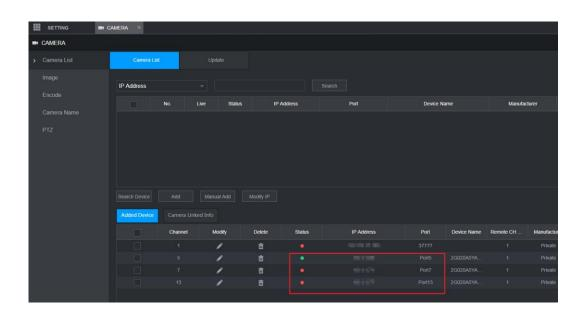
ii. When the IPC connected to POE port goes offline, the NVR will trigger an IPC offline alarm, and perform linkage operation and write an offline record to log.
