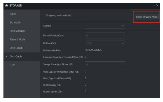
ii. Quota management allows storage capacity to be set by channel, and videos and images can be configured
