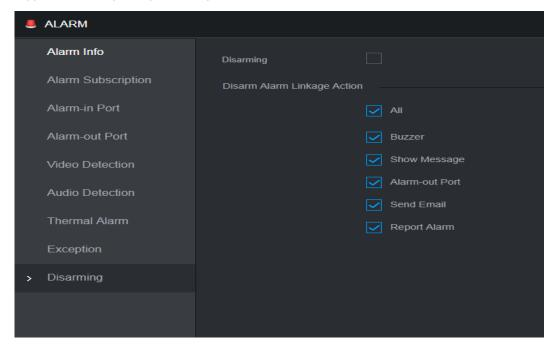
ii. The **Live** interface supports one-click disarming, and it uses a bell icon on the upper-right corner of video channels to display disarming status. When the bell is disabled, the disarming function is enabled and no alarm linkage will be triggered. When the bell is enabled, the disarming function is disabled and all alarm linkages will be triggered according to original settings.
