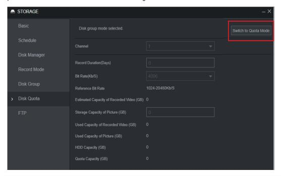
ii. Quota management allows storage capacity to be set by channel, and videos and images can be configured separately, and the remaining configurable space is automatically calculated.
