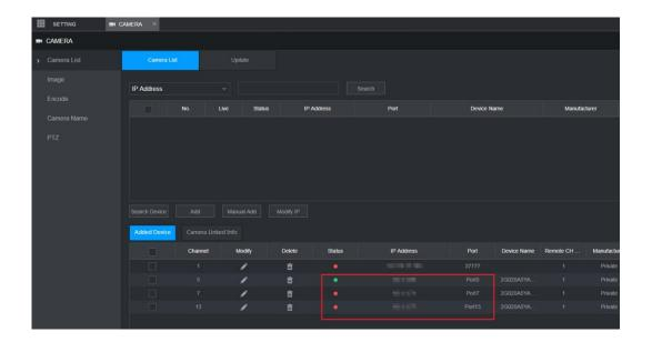
ii. When the IPC connected to POE port goes offline, the NVR will trigger an IPC offline alarm, and perform linkage operation and write an offline record to log.
