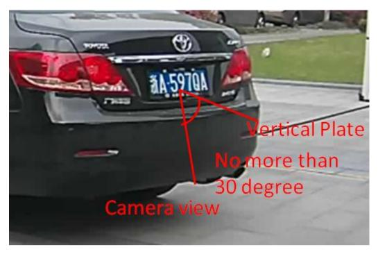
So right now the H=5m due to the position of plate is on the lane NO.2 . if we can make the monitor distance(L) longer like 8 meter, the plate angle will be smaller, but for pixels of plate maybe smaller, because the longer monitor distance, the view of camera will be bigger, so that the pixels of plate reduce.
