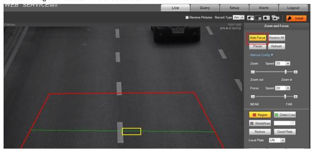
If the camera is focus manually, you can put a real plate on the camera view or focus according to the lane line of image quality at first step. Try to zoom in, focus the area you want, the result of focus will be best.
