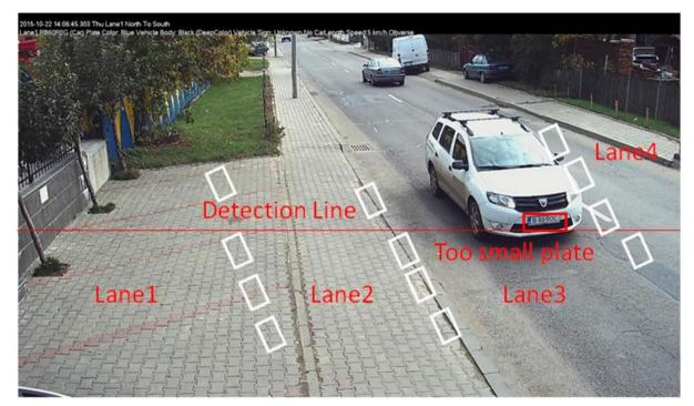
Adjust the angle of camera to shooting the road, and make the focus longer to see the plate clearly. Normally, keep the camera view as 2 lanes veiw is OK(If only need to monitor 1 lane, the camera focus can be adjusted to 1 lane- camera view)
