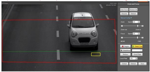
Green line means the snapshot position of detected vehicle
