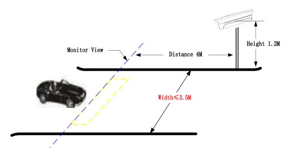
If just monitor  $4^8$  meters, the installation height of camera can be  $1^2$ meter, (detection position means the distance from camera to the vehicle detected site)
