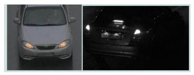
Answer: check the camera already configured to IR night mode. Or confirm the IR light if it is enough, maybe need a separate IR lamp because of the long distance.
