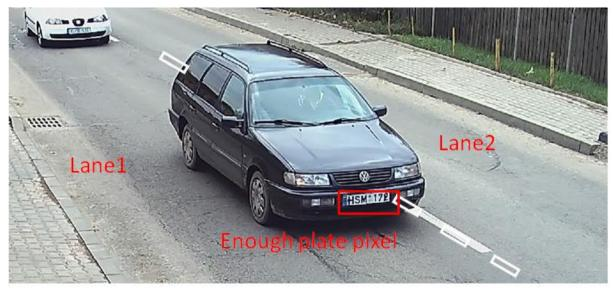
The same notification, plate should be kept as horizontal line. You can turn the camera left / right side a litter upper or down according to the plate status.
