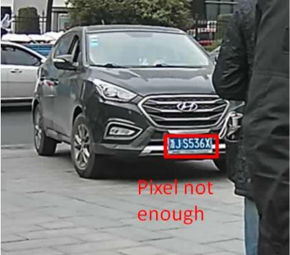
In this case, you can adjust the lens focus longer and make a more focused detection area.
