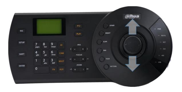
Joystick up/down: switch among different display layout, such as 1/4/6/8/9/16/25 split, etc.
