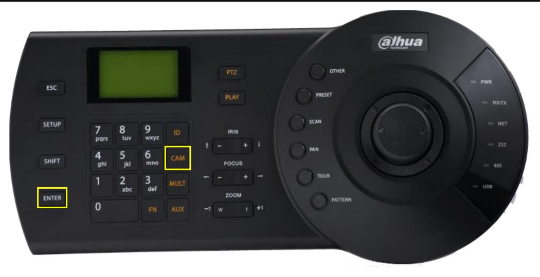
NUM + CAM: choose specific camera to display in current selected window. ENTER: switch current window between full screen and current display mode.
