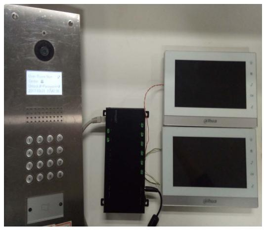
In IP 2-Wire Apartment System, VTNS1006A-2 and VTH5222CH must be used.
