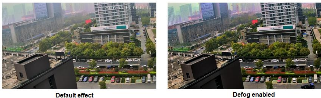
Figure 4-1 Images before and after enabling the defog mode
