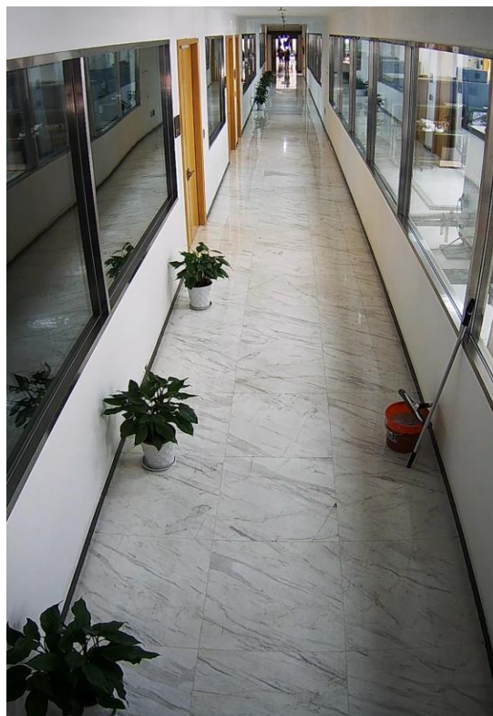
Figure 2-2 Rotate by 90° (the rotation mode) so that the monitored vertical distance is longer than the horizontal distance
