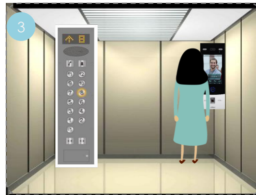
3 Light up the floor, if exceed the authenticated time, authenticate inside car again.
